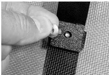
Step 14 - 15) Create metal core with screw and threaded cap
