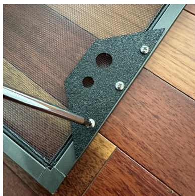
Attach Hydration mounts on the underside of the Top Screen Panel in three places
