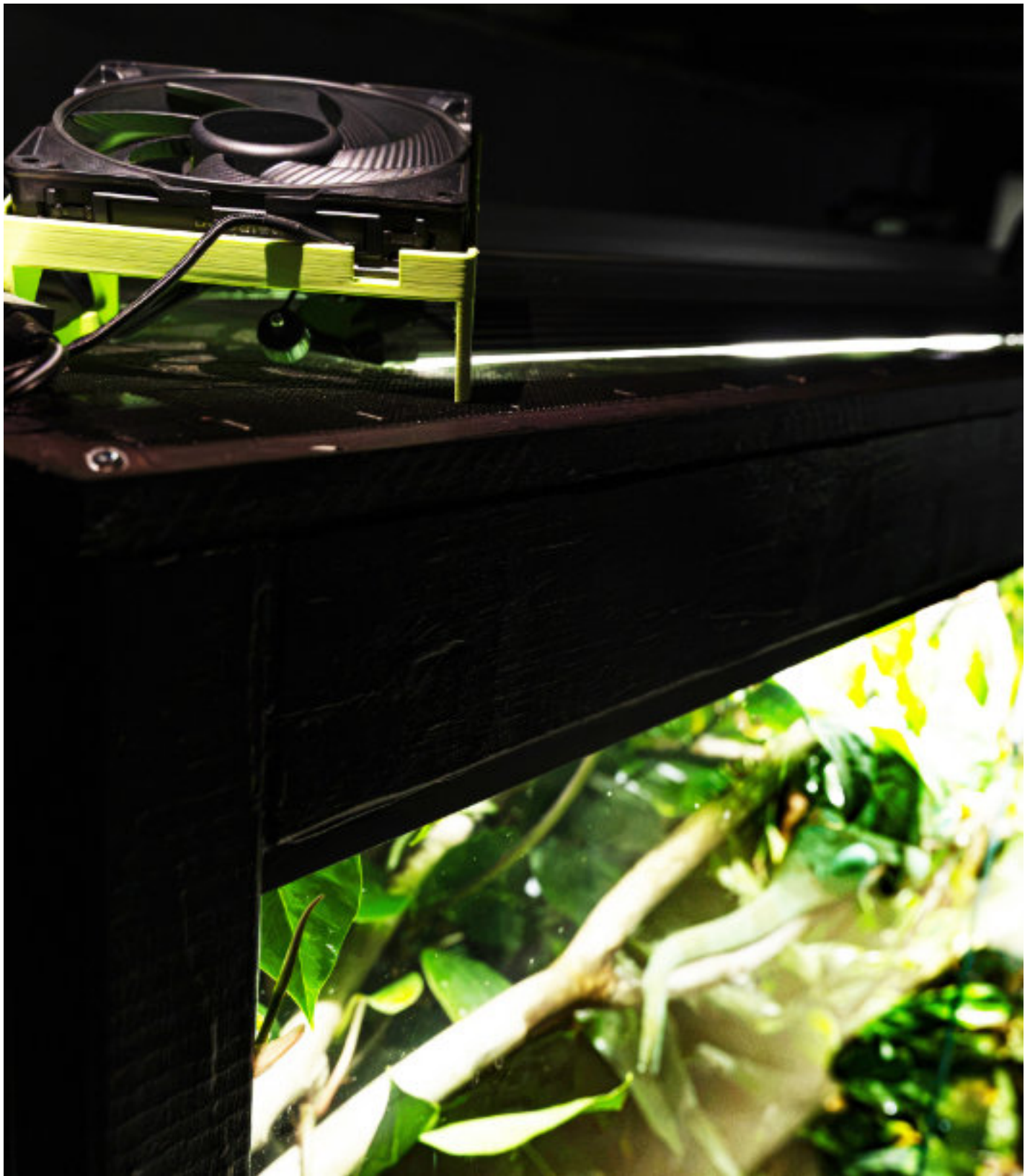
A fan clears out the warm air under the lights and the enclosure dries during the day. This custom system was designed, programmed, and manufactured by Nate Rowley. Photo courtesy of Nate Rowley
